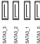
These four SATA3 connectors support SATA data cables for internal storage devices with up to 6.0 Gb/s data transfer rate.
