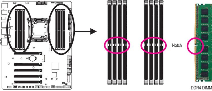
A DDR4 memory module has a notch, so it can only fit in one direction. Follow the steps below to correctly install your memory modules in the memory sockets.
