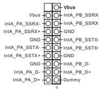
Besides two USB 3.0 ports on the I/O panel, there is one header on this motherboard. Each USB 3.0 header can support two ports.
