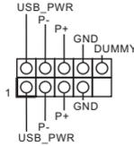
Besides four USB 2.0 ports on the I/O panel, there are two headers on this motherboard. Each USB 2.0 header can support two ports.
