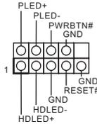
Connect the power switch, reset switch and system status indicator on the chassis to this header according to the pin assignments below. Note the positive and negative pins before connecting the cables.
