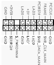
This connector supports Trusted Platform Module (TPM) system, which can securely store keys, digital certificates, passwords, and data. A TPM system also helps enhance network security, protects digital identities, and ensures platform integrity.
